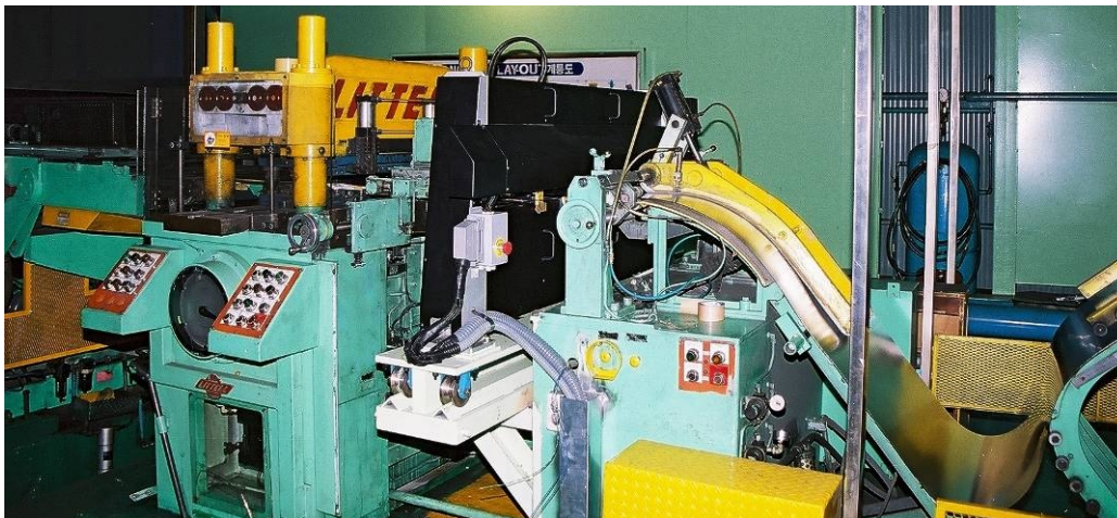
CEPHEE on a Tin Free Steel line before the shearing tool
